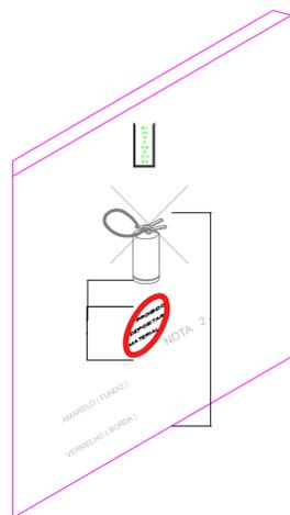
DETALHE EXTINTOR NA PAREDE
